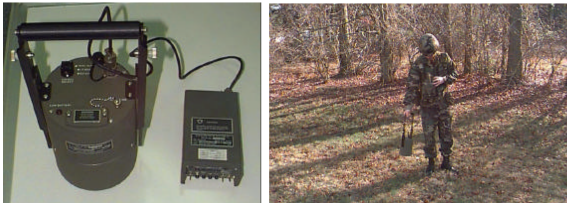
Figure 7-F: The X-Ray probe and the control unit is shown on the left. The proper use of the probe is shown on the right.
